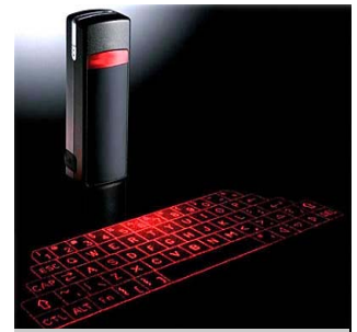
Laser projected keyboard. Image from http://
