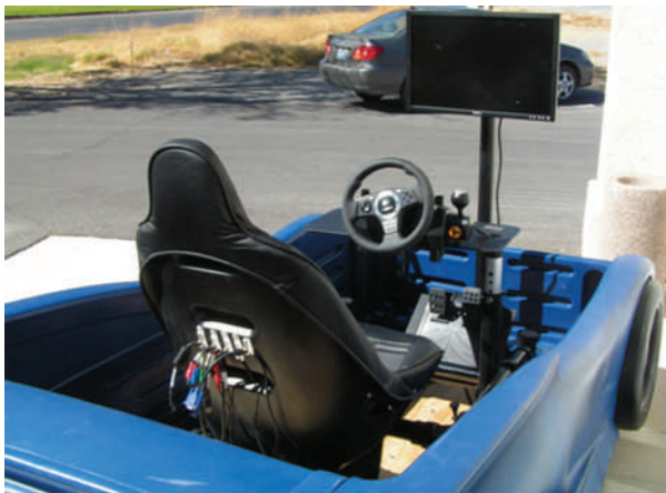
Left: The DUI Simulator mounted inside the sports car façade.
